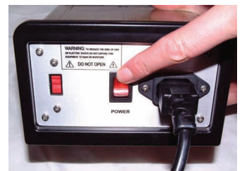
Step 8: Press the red POWER switch on the rear of the SPS power supply. A glowing red LED confirms that power is on
