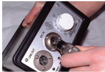
Step 2: Connect the supplied audio cable to the MIC IN socket on the front of the SPS power supply and secure the threaded collar
