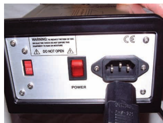
Step 7: Connect the supplied IEC mains power cable to the socket on the rear of the SPS power supply
