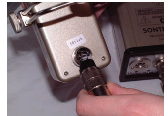
Step 4: Connect the other end of the supplied audio cable to the microphone and secure the threaded collar
