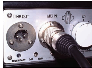
Step 3: The cable is now securely attached
