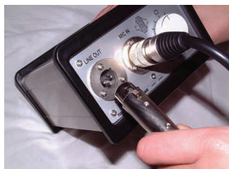
Step 6: Connect the female XLR plug to the LINE OUT socket on the front of the SPS power supply
